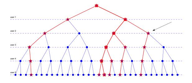
Figure 1. Tree-search algorithm for a system with N = 2 and M = 5 users and average SNR of 10 dB. The transmitted bit vector is  $\mathbf{x} = (1, -1, -1, -1, 1)^T$ . Paths with star nodes are provided by the algorithm. The final steps needs to compute 6 distances and get the minimum.
