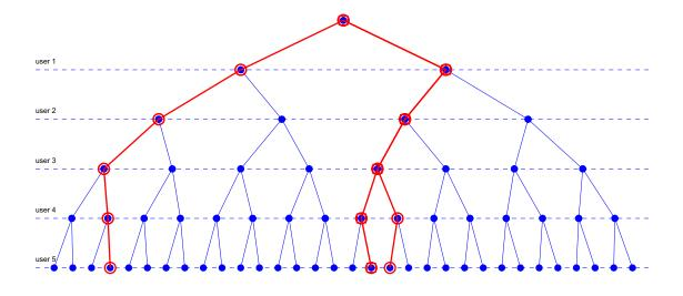
Figure 2. Two-stages tree-search algorithm for an overloaded system with N = 2 and M = 5 users and average SNR of 10 dB. The transmitted bit vector is  $\mathbf{x} = (1, -1, -1, -1, 1)^T$ . Paths with circled nodes are equilibrium points. The received signal is the same of the Fig. (1). Note the reduced number of paths that need to be considered for the final step that computes the minimum distance.
