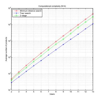
Figure 3. Average number of products for minimum distance and tree search algorithm. A system with signal space dimension N = 4 has been considered.
